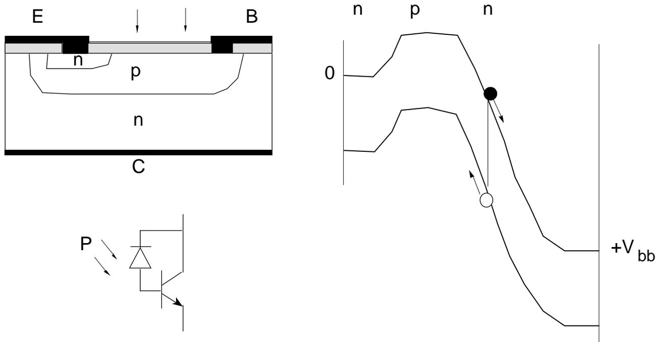
Bipolar transistor has a wide C-B junction adequate for photon dissipation, and an internal current amplification mechanism
