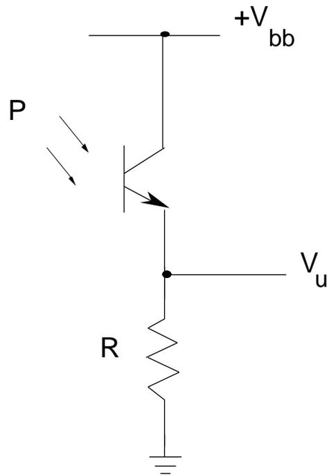
$$I_C = (h_{fe} + 1)I_{ph} + I_{CE0} + h_{fe}I_B$$
