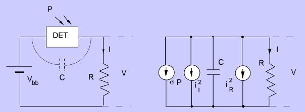
output voltage across load: $V = \sigma P \cdot R$ 3-dB high-frequency cutoff: $B = 1/2\pi RC$ noises superposed to signal : Johnson (or thermal) noise of R:
