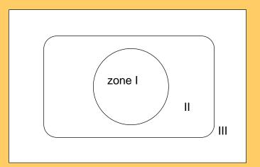
In zones I, II, II, a top quality (Aclass) tube may have 0, 1, 3 defects not larger than 1 pixel, a class B 1, 3, 10 and a industrial-class (Xclass) 5, 20, >20.
