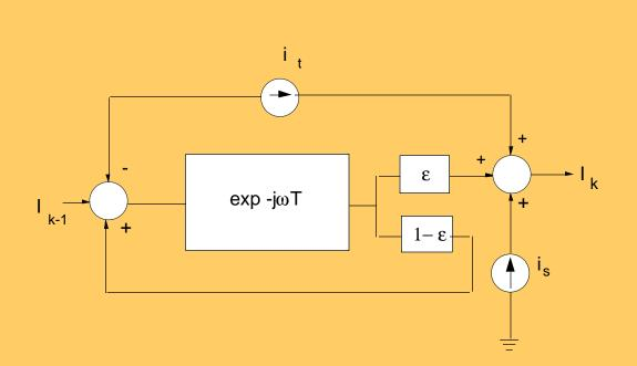
k-th cell is schematized by a delay T (clock phase), a transfer inefficiency  $\varepsilon$  and shot-noise generators  $i_t$  (transfer) and  $i_s$  (storage)
