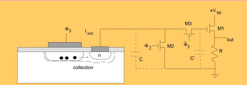
noise:  $v_n^2 = 2e[FI_{ph} + 2nI_d]B R^2 + (8/3) kT B/g_m + kT/C + 4kTBR$  $\approx 2e[FI_{ph} + 2nI_d]B R^2 + (8/3) kT B/g_m + kT/C$  (for  $g_m R >>1$ )
